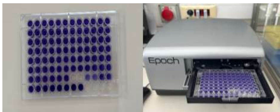
Figure 3. Measurement of FRAP activity at 593 nm following incubation
