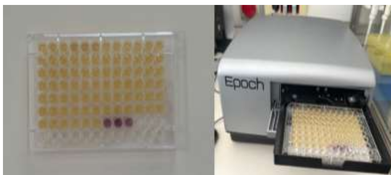
Figure 2. Absorbance measurement at 515 nm for the DPPH assay using a microplate reader
