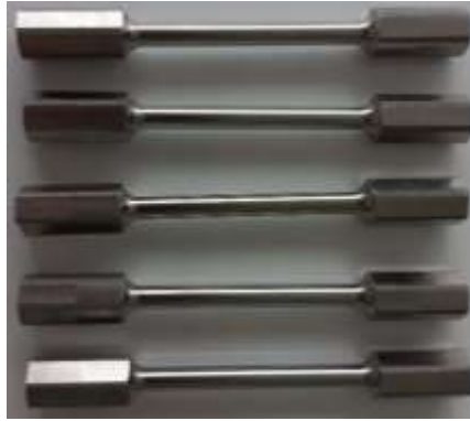
Figure 2. Torsion test specimens machined with turning
