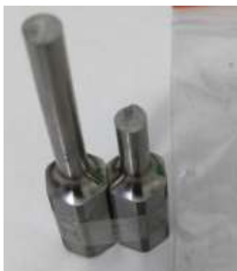
Figure 7. Sample after torsion test
